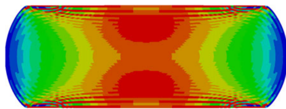
(b) Example of the checkerboarding spatial instabilities (hydrostatic pressure field) in cell-centred finite volume formulations (taken from [30])
