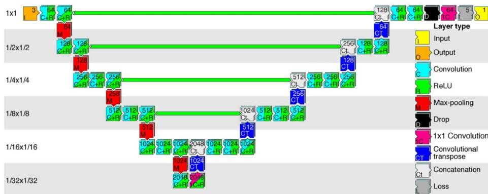
Fig. 5 CNN design used in [84], which was based on the U-Net model
