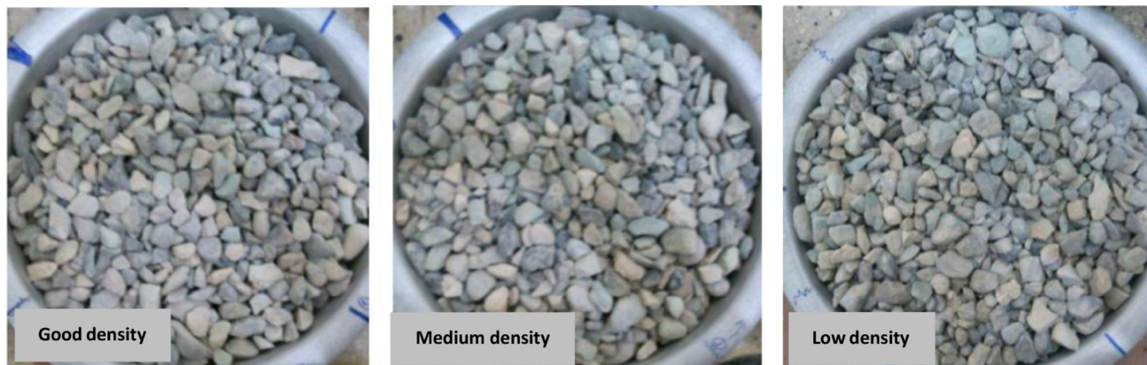
Fig. 12 Some aggregate samples at different density
