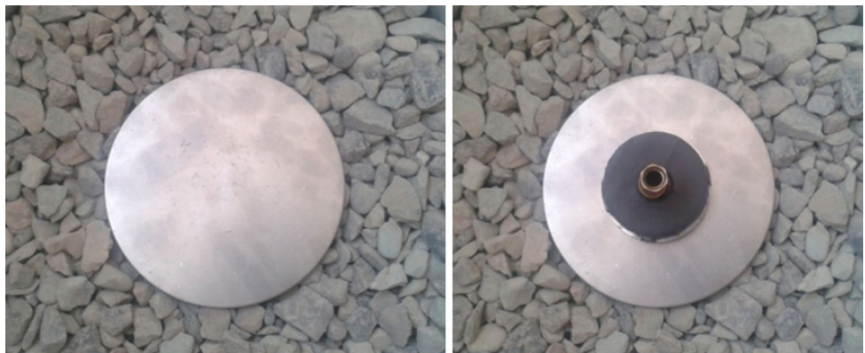
Fig. 8 The steel plate is placed on aggregate. Then, the sinker is released on the steel plate
