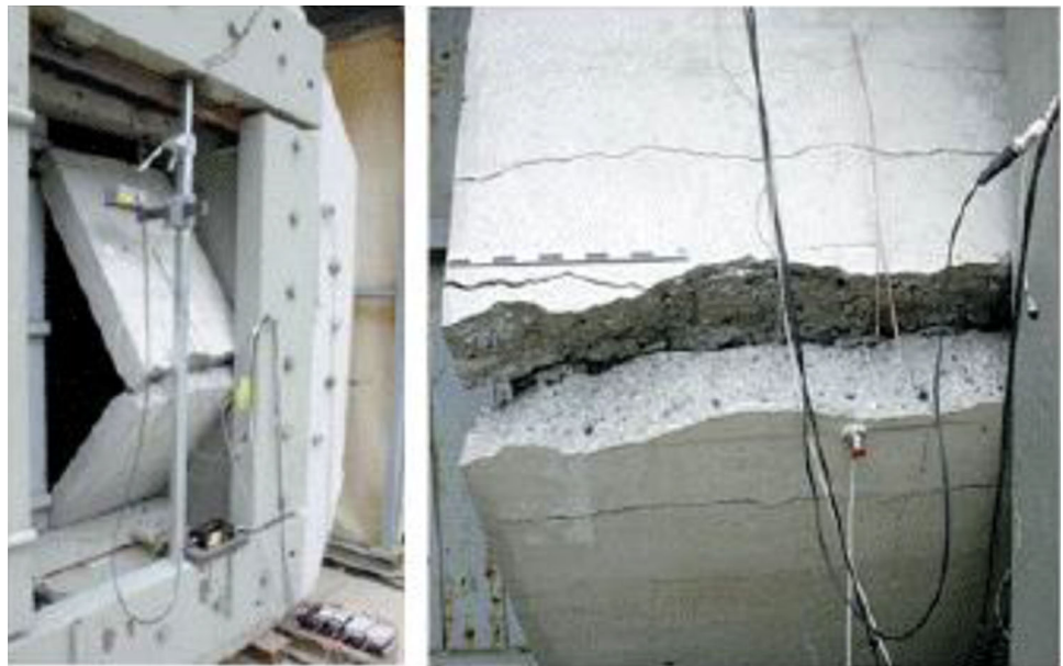
Fig. 13 Result from a shock tube test of a RC panel in [74]
