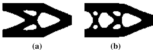
Fig. 49 Design of two-scale structures in nonlinear elasticity for two different loading cases: a f_{ext} = 0.01 N, b f_{ext} = 0.2 N [149]
