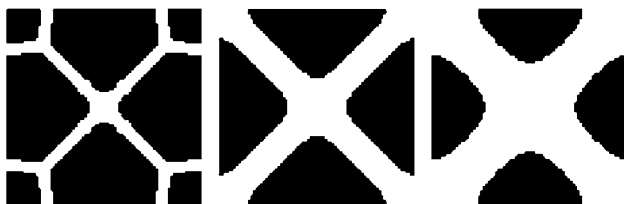
Fig. 37 Optimized results for maximizing damping of composites made of stiff elastic phase ( black ) and soft viscoelastic phase ( white ) where the volume fractions of viscoelastic phase are 20, 40, 60% and corresponding loss tangents are 0.53, 0.61, 0.64 from left to right , respectively [64]
