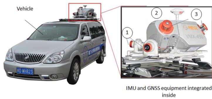
(c) 1-Digital Camera 2-GNSS Antenna 3-Laser Scanners
