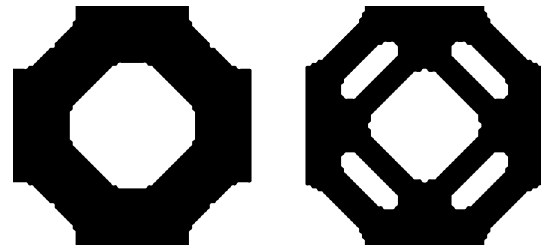
Fig. 14 Microstructures with maximized shear moduli obtained using filter radii 12 mm (left, shear modulus 0.1688 MPa) and 8 mm (right, shear modulus 0.1746 MPa)
