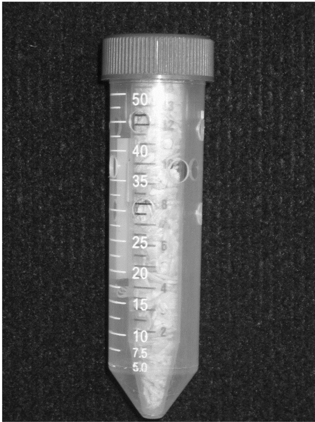
Fig. 1 Wireworm probe trap (prototype) comprising outer collection tube (50 ml centrifuge tube) and an inner bait barrel (15 ml centrifuge tube), the latter containing 4.5 g rolled oats to generate carbon dioxide by aerobic fermentation
