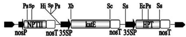
Fig. 1 Structure of the T-DNA region of pIG121-Hm/ katE . Ec Eco RI, Hi Hind III, Ps Pst I, Sc Sac I, Sn Sna BI, Sp Sph I, Ss Sse I, Xb Xba I, NPTII neomycin phosphotransferase II, HPT hygromycin phosphotransferase
