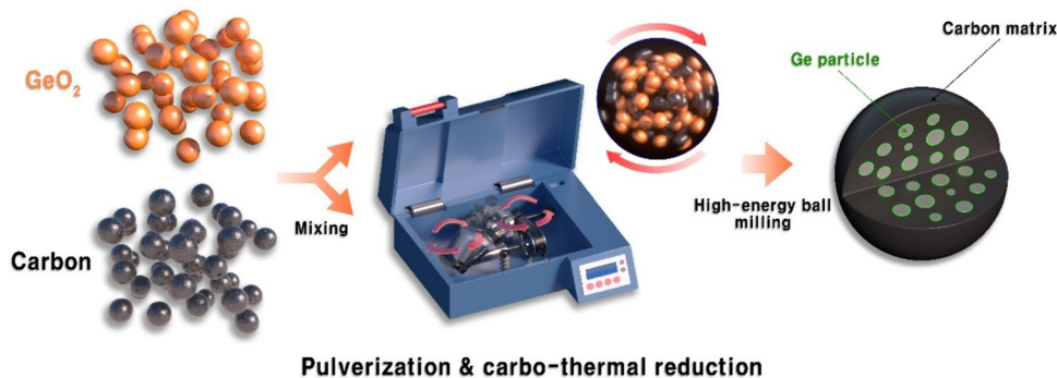
Fig. 1 Schematic illustration of high-energy ball milling for synthesis of the Ge@GeO 2 -C composite material
