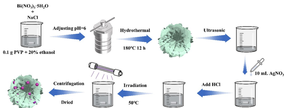
Fig. 1 The schematic illustration of Ag/AgCl/BiOCl hetero-junction synthesis process
