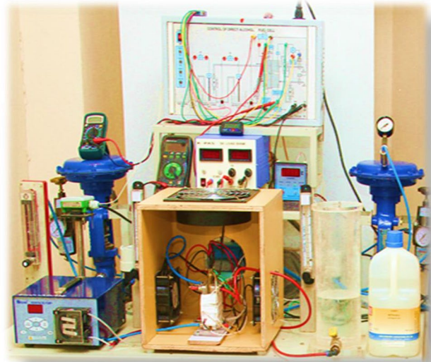
Fig. 3 Real-time laboratory experimental setup of DMFC control system
