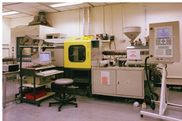
Fig. 1. Photo of the injection molding machine at HKUST's Advanced Materials Lab.
