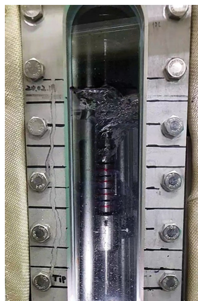
Fig. 4. Vortex and surface height image taken using the high-speed camera for base impeller position.
