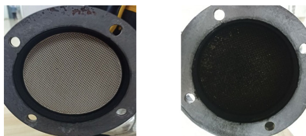
Fig. 1. Contrast of the GPF-B without soot loading and with soot loading.
