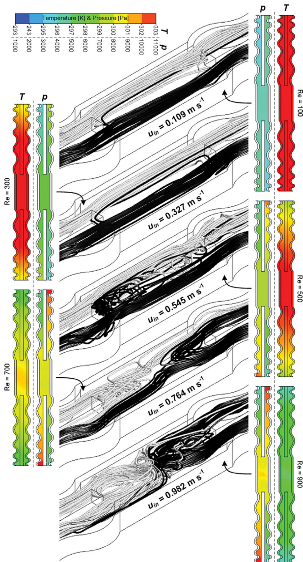
Fig. 7. Effects of inlet velocity on pathlines, temperature distribution on base surface, and pressure distribution on certain plane of y=1.5 mm inside WSW3.
