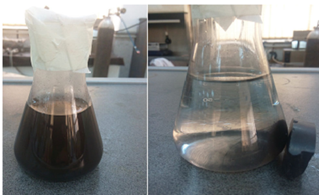
Fig. 6. Draw solution ( \text{Fe}_3\text{O}_4 nanoparticle) before and after applied magnetic field.
