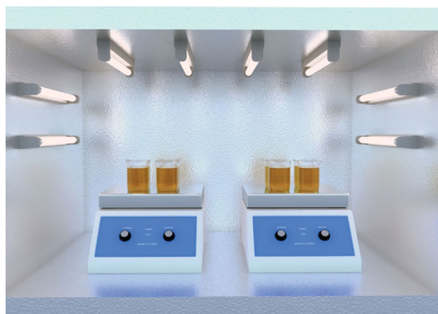
Fig. 1. A schematic representation of Photo-Fenton process.
