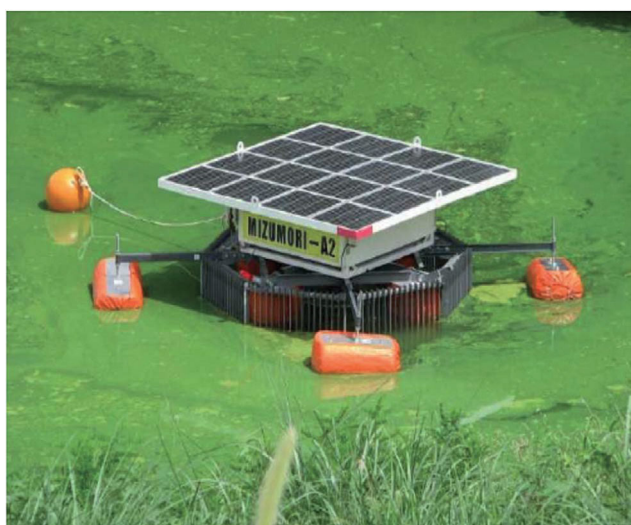
Fig. 15. Photograph of a self-propelled liquid phase plasma apparatus floating over a dam to destroy the harmful Microcystis aeruginosa . Reproduced from ref. [59]. Copyright Kumamoto University, Japan.
