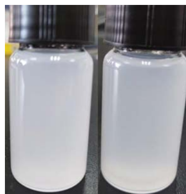
Fig. 3. Photograph of PNHAs dispersed in DMAc solution before (left) and after (right) standing for 1 day.
