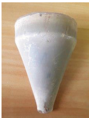
Fig. 4. Conical shell produced by electroforming method.
