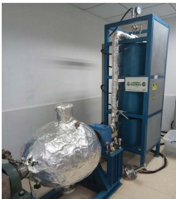
Fig. 1. Ball-shaped reactor for the production of cellulosic pulp by CAOSA process.
