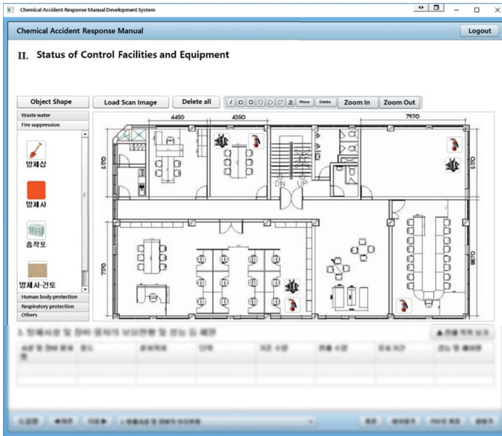
Fig. 4. Facility floor plan and equipment status screen.
