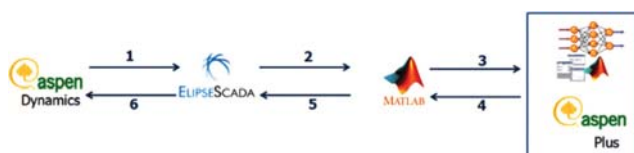
Fig. 4. Communication between used software programs.
