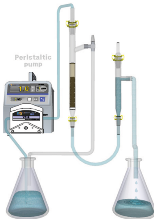
Fig. 2. Schematic diagram of column-type packed-bed adsorption reactor.
