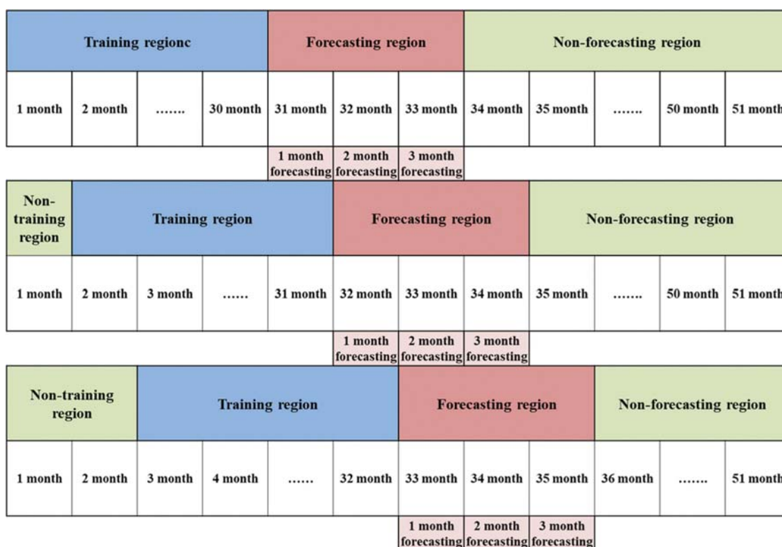
Fig. 9. Time window movement for the forecasting of the naphtha crack.
