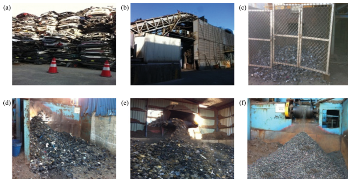
Fig. 1. Products from shredding process. (a) Compressed vehicle fluff. (b) Shredding vehicle fluff. (c) Non-ferrous metal. (d) Heavy fluff. (e) Light fluff. (f) Glass & soil.
