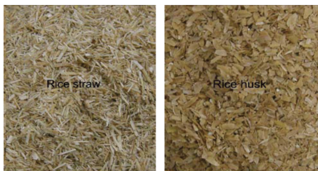
Fig. 1. Images of rice straw and husk used for the fabrication of pellets in our study.
