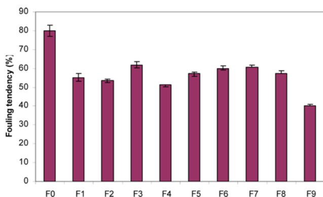
Fig. 9. Fouling tendency of the prepared thin layers.
