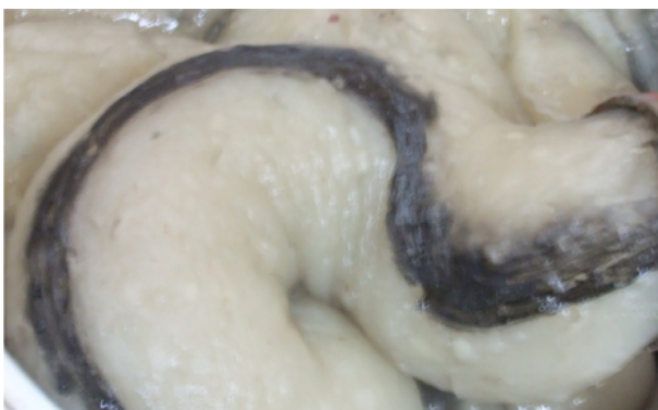
Fig. 13. Poor mixing at Re=16 .
