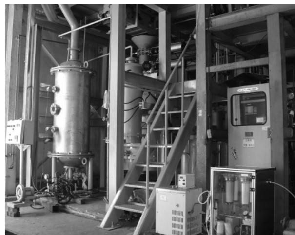
Fig. 2. View of the gasification system including a reformer using high-temperature air.
