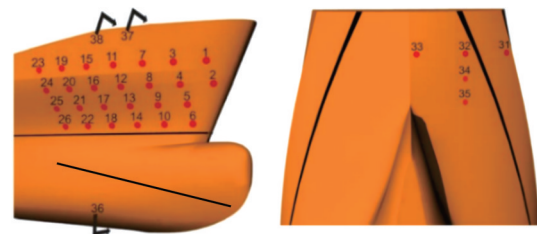
Figure 2 Overview of pressure transducer locations
