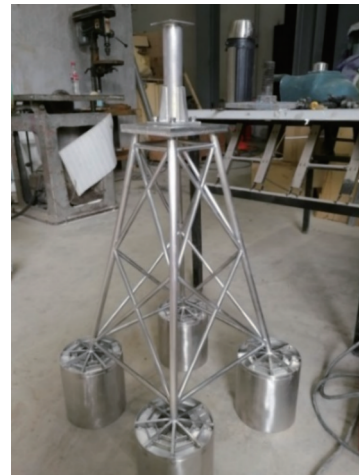
Figure 2 Test model of the four-bucket jacket foundation
