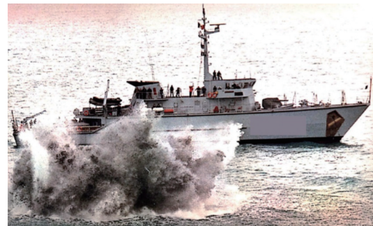
Figure 5 Underwater shock test explosion (MARIPERMAN, 1988)
