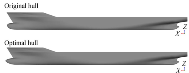
Figure 21 Comparison of the parametric hull and the optimal hull for the KCS at design speed
