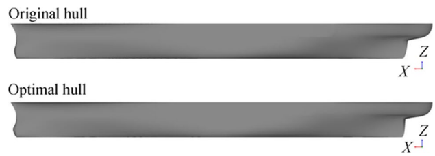
Figure 27 Comparison of the original hull and the optimal hull for the S-175 at Fr = 0.250
