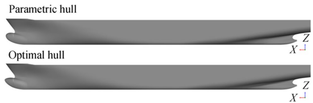
Figure 15 Comparison of the parametric hull and the optimal hull for the DTC at design speed
