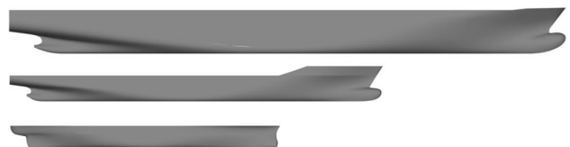
Figure 1 Original hull forms of the DTC (top), the KCS (center), and the S-175 (bottom)
