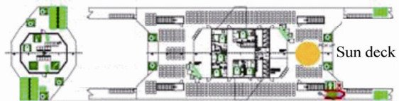
Fig. 13 Sun deck: Relocation of the helicopter pick up area
