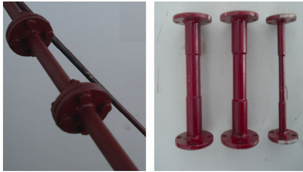
Fig. 17 Flange members replaced to simulate damage
