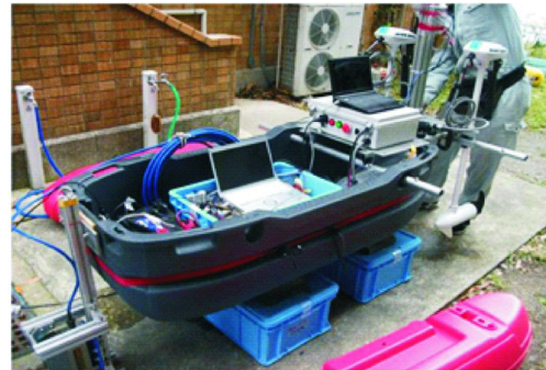
1. Imagenex™ DeltaT multi-beam sonar with stainless guard; 2. thruster (left; viewed from astern)
