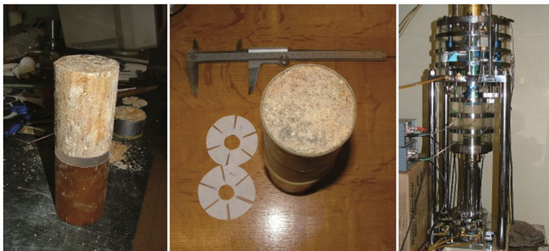
Fig. 9 Soil specimens for RC testing
