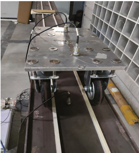
Fig. 7 Instrumentation on model car and bridge model with accelerometers
