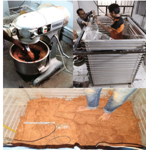
Fig. 4 Preparation of clay soil
