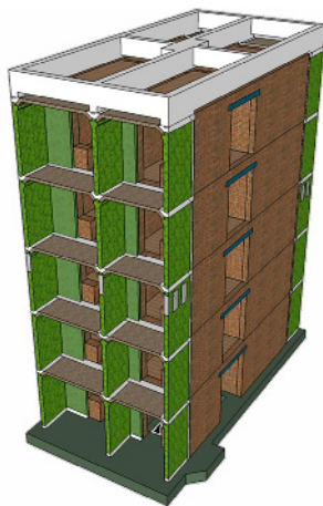
Fig. 1 Full-scale five-floor retrofitted masonry building
