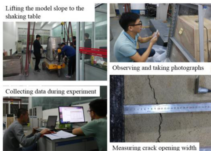
Fig. 3 Partial shaking table test procedure
