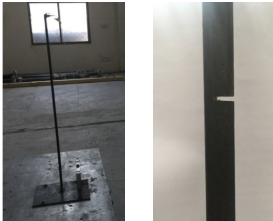
Fig. 2 Zoom view of undamaged and structure damaged column for experimentation
