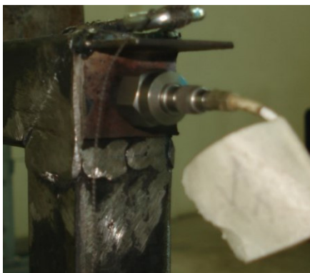
Fig. 12 Zoom view of accelerometer attached to the top end
