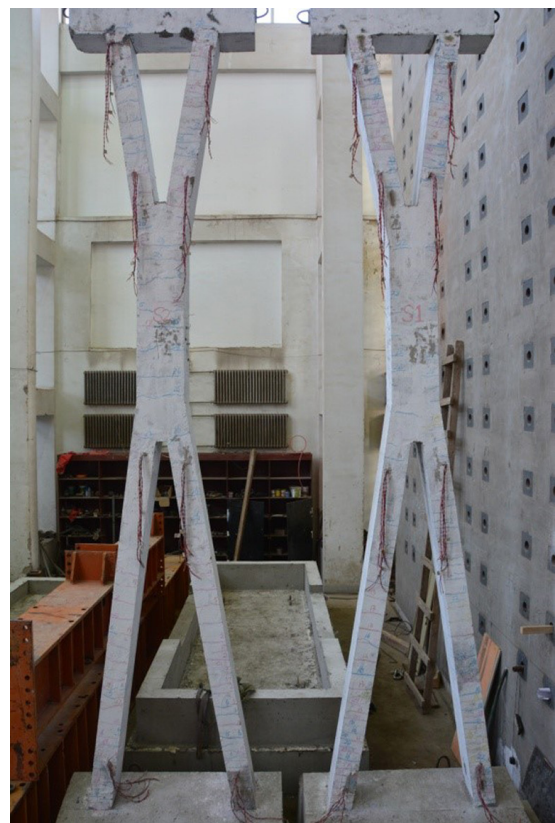
Fig. 31 Damage of the two specimens
