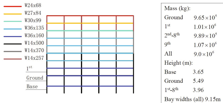
Fig. 1 Nine-story steel structure YZ moment-resisting frame of the benchmark building (The first three periods of the model are: T_1 = 2.28 s, T_2 = 0.828 s, T_3 = 0.4463 s)
