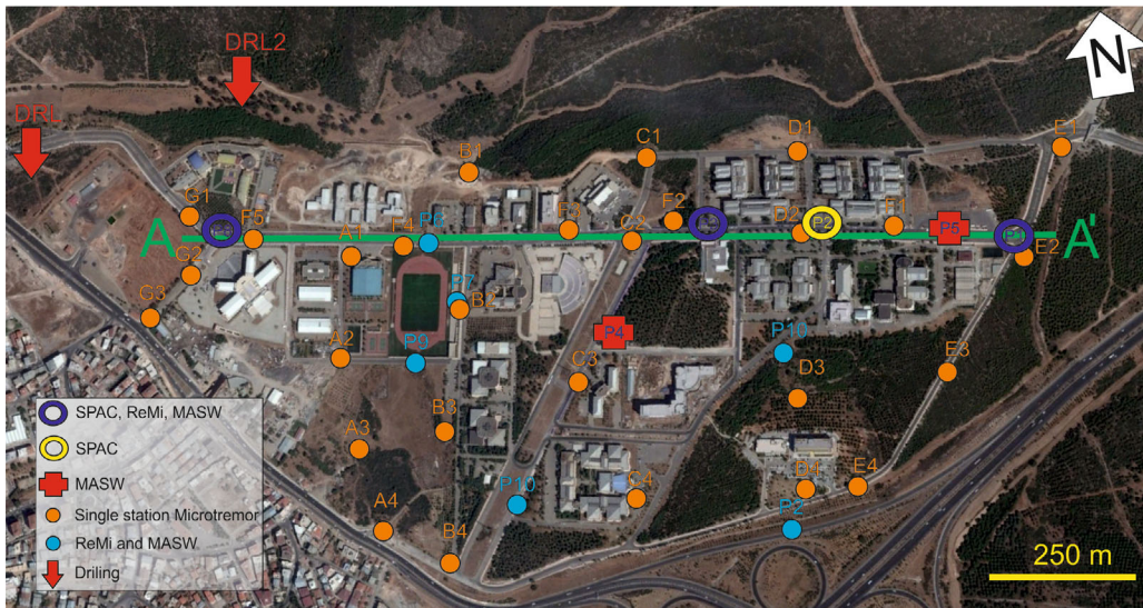
Fig. 4 Map of the study area with the locations of the 28 sites of the microtremor measurements and 11 sites of V_s measurements
