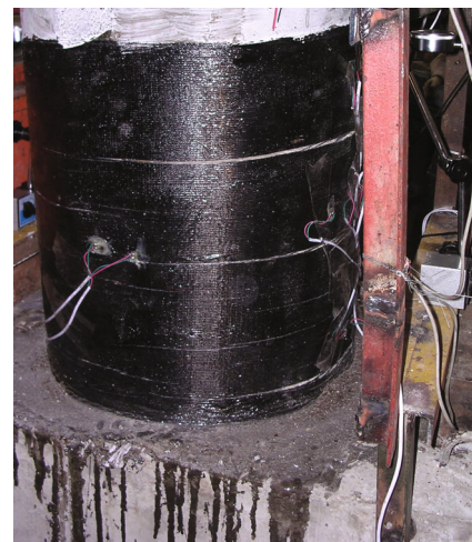
Fig. 10 Flexural cracks of CFRP sheets in specimen A14-R
