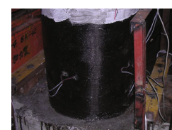
(e) Specimen A14 after wrapping of CFRP
