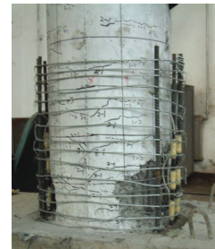
(c) Specimen A12 after additional longitudinal and spiral bars are arranged
