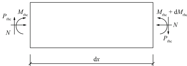
Fig. 17 Force diagram of specimen for bond failure
