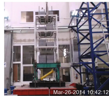
(b) Three-story \frac{1}{4} scale test model on the shake table
