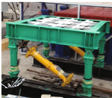
(a) Seismic isolation story
